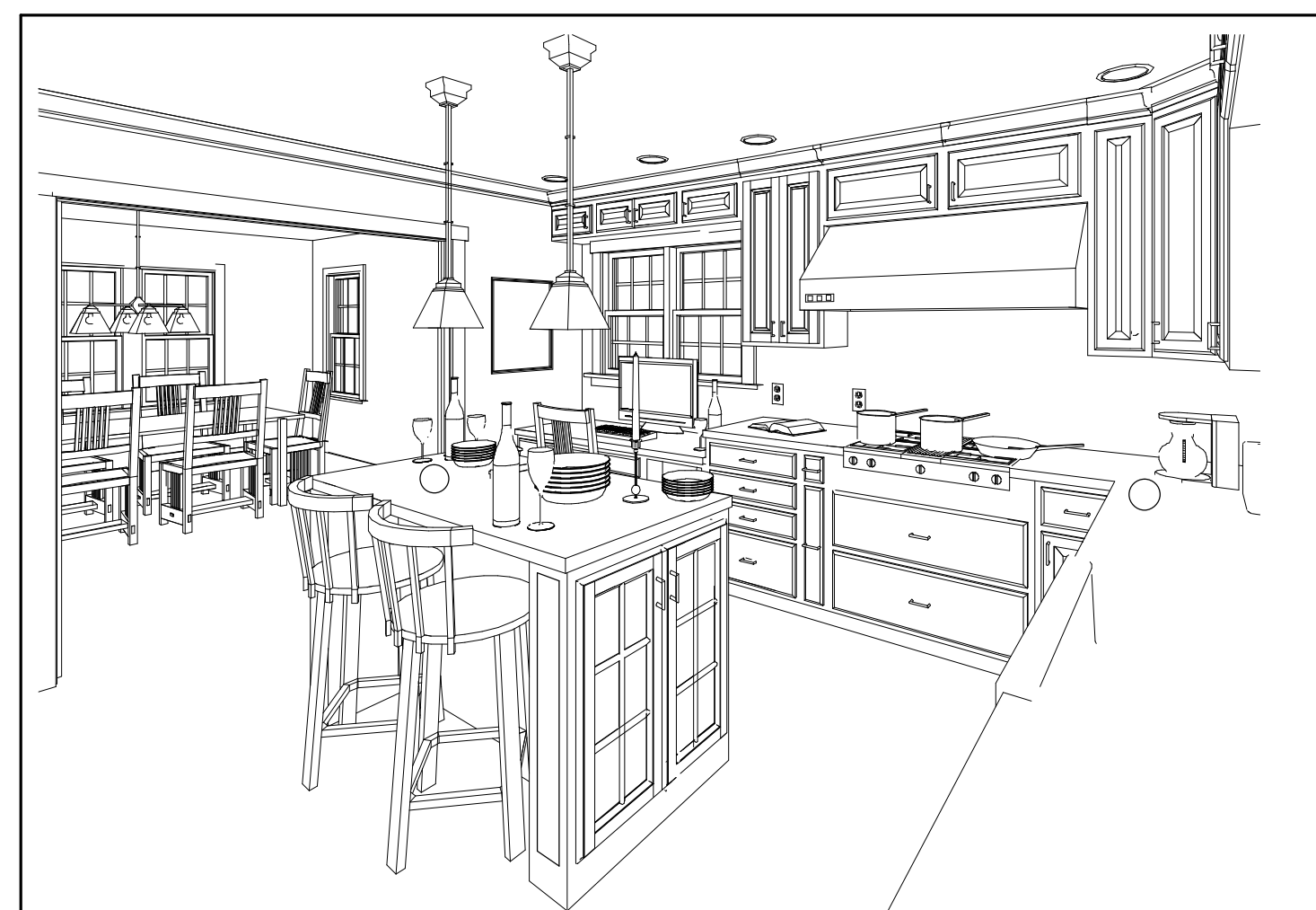
C GAS STOVE W/ POT STORAGE DRAWERS BELOW FRENCH DOORS TO DINING AREA BEYOND
