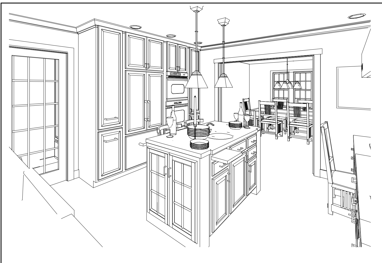
B CENTER ISLAND WITH SINK AND PULLOUT BUTCHER BLOCK PULL OUT PANTRY /OVEN / MICROWAVE REF./FREEZER BEYOND
